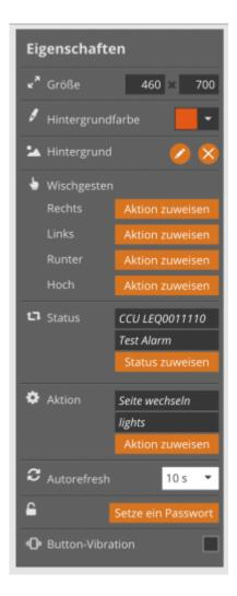
Similar to buttons it is possible assign a status to a page and additionally an expected target value. Click on a free space on the remote page and then in the settings panel to the right on "Assign Status".
