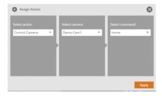
When pressing the button the assigned action (i.e. panning the camera to the left) will be executed.  $\rightarrow$  Doorbird: available actions  $\Rightarrow$  "open door" and "light on".
