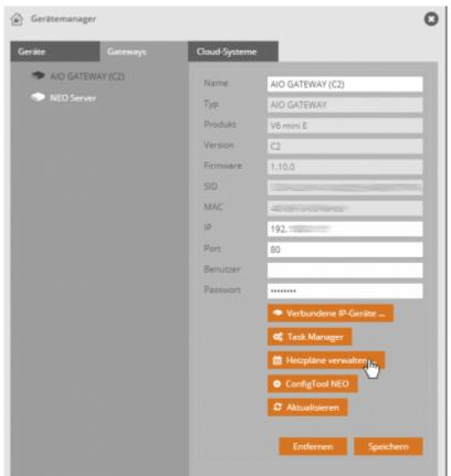
To create a heating plan, open the tab *Gateways* in Device Manager and select your AIO GATEWAY. Choose here *manage heat plans*.
