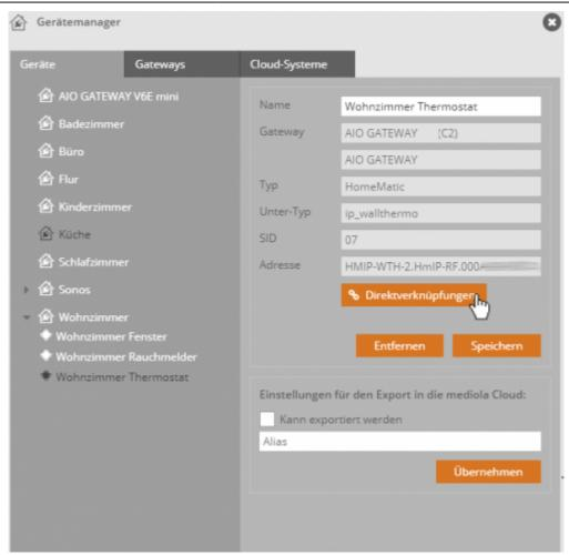
Direct links are created in the device manager in one of the two devices to be linked. Open the device manager and go to one of the devices you want to link. Click on *Direct Links* .
