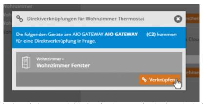
You will now see all devices that are available for direct connection to the selected device. Click *Connect* to create the direct link to this device.
