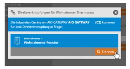
To undo a direct link, go to the corresponding device in the device manager and click on *Direct Links*. The linked device is then shown with a blue background. With *Disconnect* you can disconnect the created direct link.
