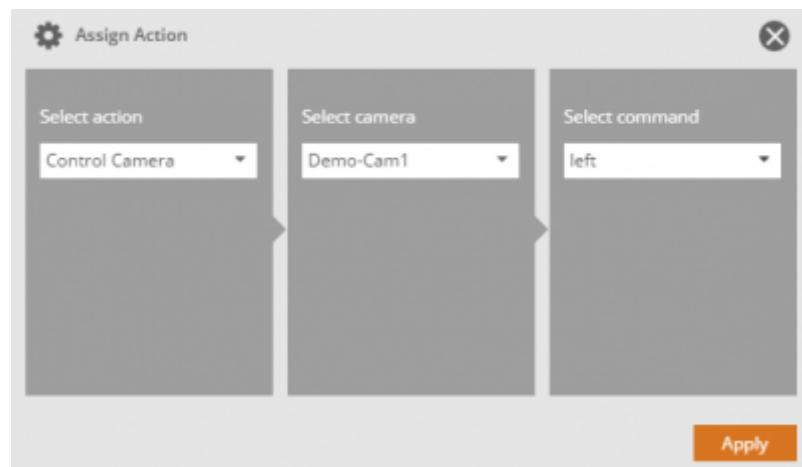
Tapping the button will execute the assigned command (i.e. turning a pan/tilt camera).
