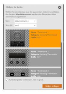
After adding the widget to the remote page, the functions of the selected device (Actions / Status) are already assigned to any single element of the widget. Now the widget can be edited like a normal group element (i.e. resize, ungroup, etc.). If you want to change the layout of the widget, it is necessary to ungroup the widget group in the properties with the command "Disband Group".
