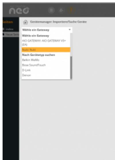
Now NEO displays the devices paired with the NUKI BRIDGE. Select the devices you want to import by checking the box. Finally click on "Import".
