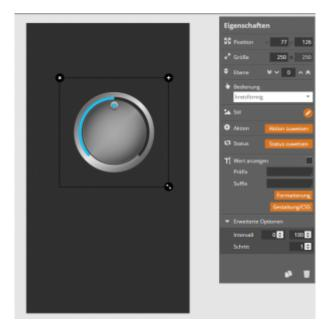
An action and / or a status can be assigned to the slider in the properties menu on the right. In addition, the operator can set whether the slider should react to a circular wiping movement or a linear movement from left to right. The display of the values is optional and can be activated by ticking the appropriate box. The text can be formatted using CSS.
