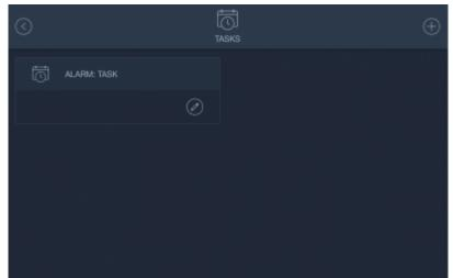
On the V6-Series gateways an alarm task is automatically created and indicated by **Alarm:**. Go to main menu -> tasks to define your alarm task individually. The process is similar to normal tasks. Check the chapter tasks for more information about how to define triggers and actions.
