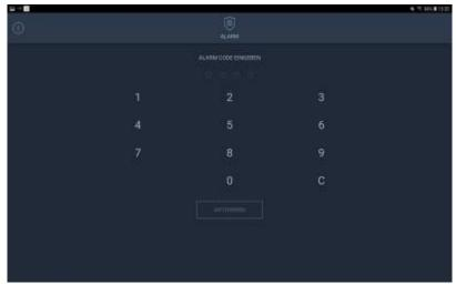
To activate/ deactivate an alarm task in IQONTROL NEO, tap on the *Alarm* button on the dashboard. Then enter your 4-digit alarm PIN and tap *activate* or *deactivate*. The status of your alarm task is indicated on the *Alarm* tile as shown below:
