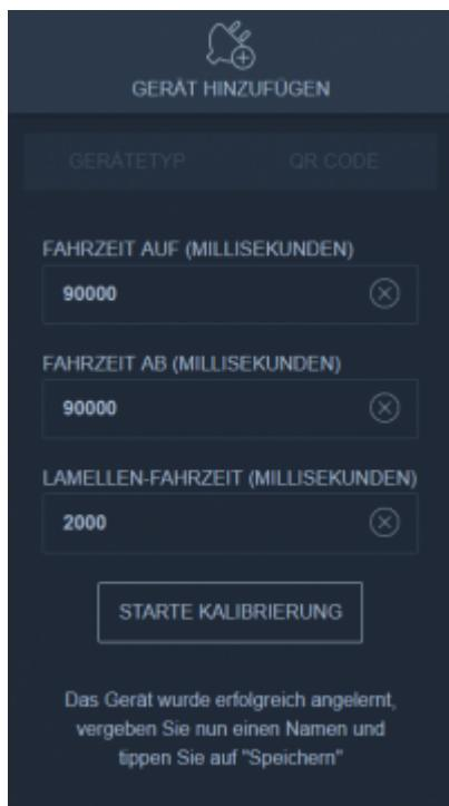
The travel time is specified here in milliseconds for up and down (and, in the case of blinds, also for slats). The roller shutter is automatically adjusted to match via \* Start calibration \*.
