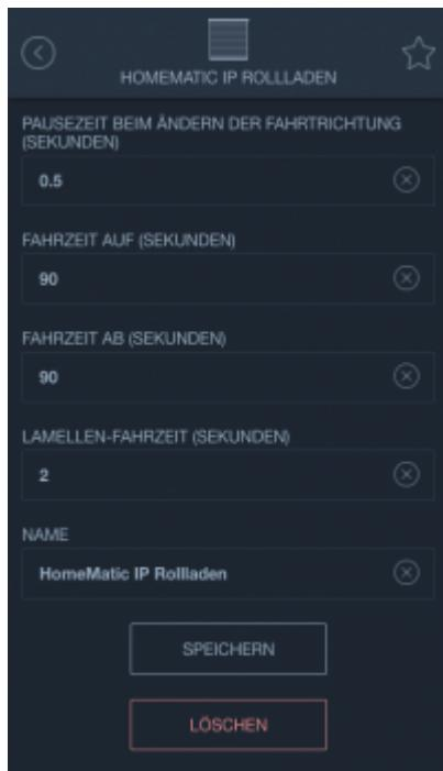
There is no difference between Homematic and Homematic IP. Set the travel time for \* Up \* and \* Down \* in seconds and, in addition to the slat travel time (blinds only), also set the pause time for changing the travel direction.
