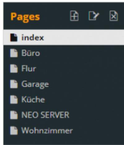
Each remote page basically consists of a background and various elements (eg buttons, sliders, text fields), which can be positioned on it freely. To design and modify a remote page in the editing area you have to select it in the remote page list.
