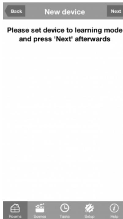
Then press “Next”. The actuator is now paired with the gateway. The “prog” and rf led start flashing red and orange in turn. Once the spinner in the app is removed the pairing process has been finished. Again follow the instructions on the screen and quit the teach in process on the actuator by pressing the plastic pin in the “Prog” hole once. When done press “Next”.
