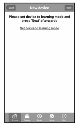
If a blind has been programmed by an original remote control to the shutter please set the remote in learning mode. You can do this by pushing onto the button until the shutter gives you a feedback by shortly moving up and down. Now you have to tap on "Next". After the programming has been successful the blind will give again a feedback by shortly moving up and down. The gateway is now programmed as an additional remote.
